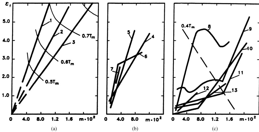
Fig. 2. Effect of the strain-rate sensitivity on the fracture strain in the tensile test over the test temperature range 0.1–0.8  $T_m$  for: (a) face-centered cubic metals: (1) silver, (2) copper, (3) aluminium; (b) body-centered cubic metals: (4) iron, (5) vanadium, (6) molybdenum, (7) chromium; (c) hexagonal close-packed metals: (8) cadmium, (9) titanium, (10) zinc, (11) cobalt, (12) magnesium, (13) lanthanum.
