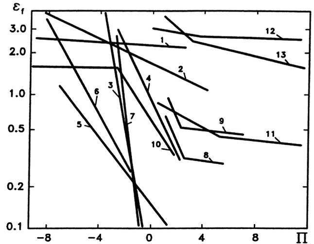
Fig. 3. Effect of the  $\Pi$ -factor on the fracture strain: (1) niobium, (2) iron, (3) tungsten, (4) molybdenum, (5) beryllium, (6) magnesium, (7) zinc, (8) tin alloy, (9) brass, (10) brass alloy, (11) tin bronze, (12) deformed lead, (13) cast lead.
