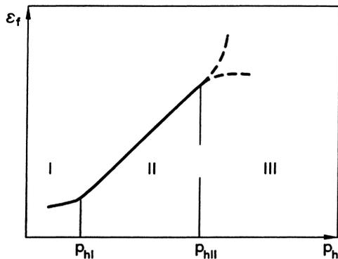
Fig. 5. Generalized dependence of the fracture strain  $\epsilon_f$  on the hydrostatic stress  $\sigma_m$ .
