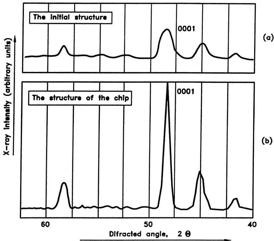
Fig. 7. Diffractometer traces of the titanium alloy: (a) the initial structure; (b) the structure of the chip.
