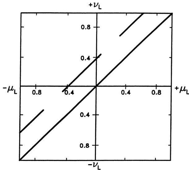
Fig. 4. Diagrammatic representation of the Lode parameters for ideal plastic (---) and strain-hardening (—) materials.
