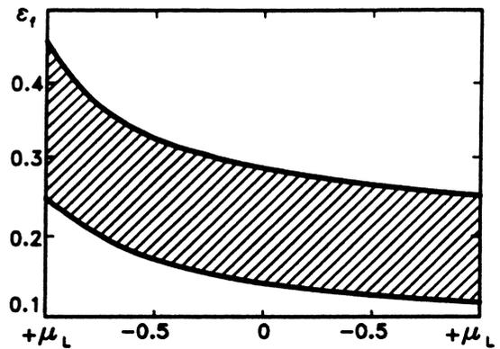
Fig. 6. Changes in the effect of the Lode stress parameter on the fracture strain.
