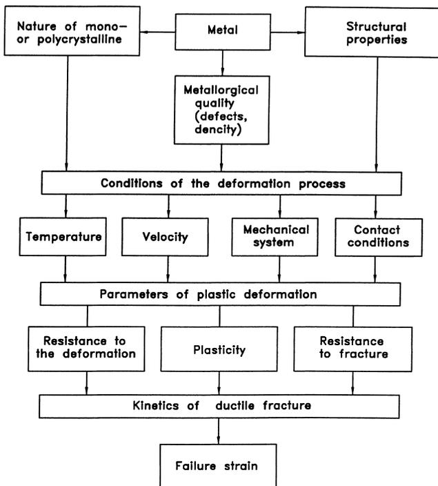
Fig. 1. Major interactions between the fracture strain and other structural-deformation parameters.
